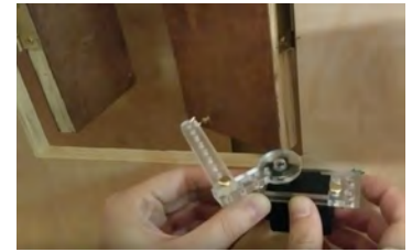
Creating the mechanism for the door to open using the servo. Testing the device.
