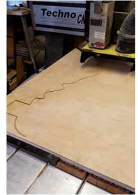
Two clocks were fabricated using plywood and cut on the CNC machine.
