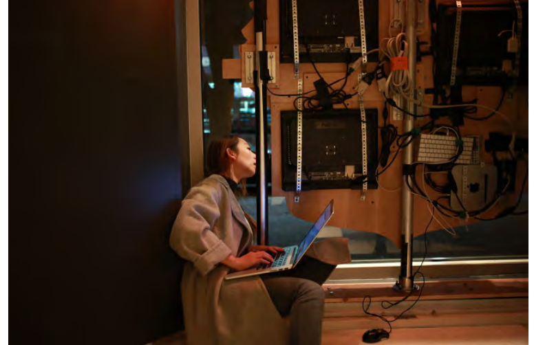
Setting up the system. Wires, mac mini and monitors secured. Base of the clock is fastened to the shallow window to prevent tilting.
