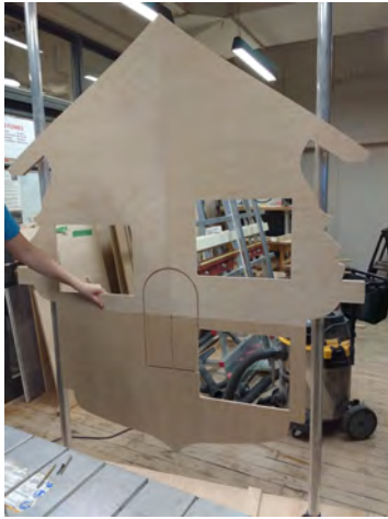
Each clock comprised of three parts, which were later connected at the back. Each clock was fastened to two steel poles and a wooden base.
